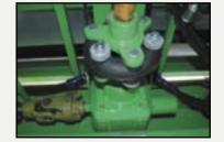
The mechanical angle transmission is protected by 2 anti-torsion silentblocks absorbing the shocks turning up when starting to unload.
