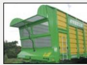
The quick-opening side door turns out to be very useful for maintenance and cleaning operations
