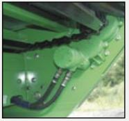
The two hydraulic motors (protected under the floor) making the floor move are fitted with two gears. The first gear allows to start the moving floor and progressively increase its speed. Then, the second gear makes it possible to unload the silage trailer quickly and regularly.
