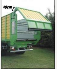
The silage trailer is unloaded easily and without blocking thanks to the significant rear door off-set (about 40 cm) above the body. The rear door is operated by 2 double-acting cylinders. The rear door is also equipped with a locking spring system.
