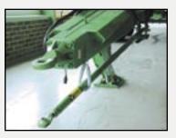
The steering cylinder is controlled by a sensor cylinder clamped to the drawbar by means of a knee-joint. The system is balanced thanks to the compensated cylinders, which exert a similar force in both directions. The circuit is fitted with a onepiece set-up unit consisting of one pressure gauge, two nitrogen accumulators, one balancing valve and one calibration system.
