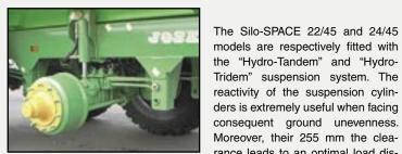
models are respectively fitted with the "Hydro-Tandem" and "Hydro-Tridem" suspension system. The reactivity of the suspension cylinders is extremely useful when facing consequent ground unevenness. Moreover, their 255 mm the clearance leads to an optimal load distribution in all circumstances. In option, the 20/40 model can also be equipped with the "Hydro-Tandem" suspension
