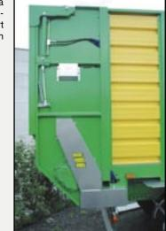
The 20/40 and 22/45 models are equipped with an adjustable drawbar with cross-springs.
